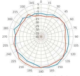
5.5 GHz Wi-Fi average elevation 05.5 GHz Wi-Fi average elevation 90
