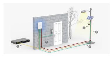
**Port 1:** 24/48V DC 4 Pair Passive PoE Camera **Port 2:** 802.3af PoE IP Video Intercom System
